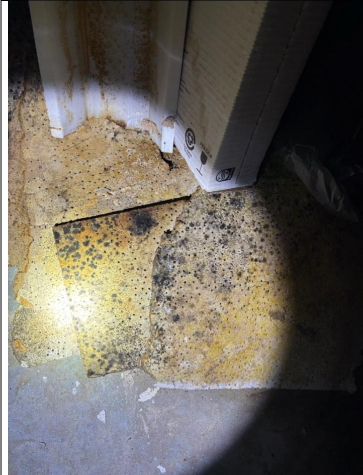
Fungal growth observed on stored building materials in basement.
